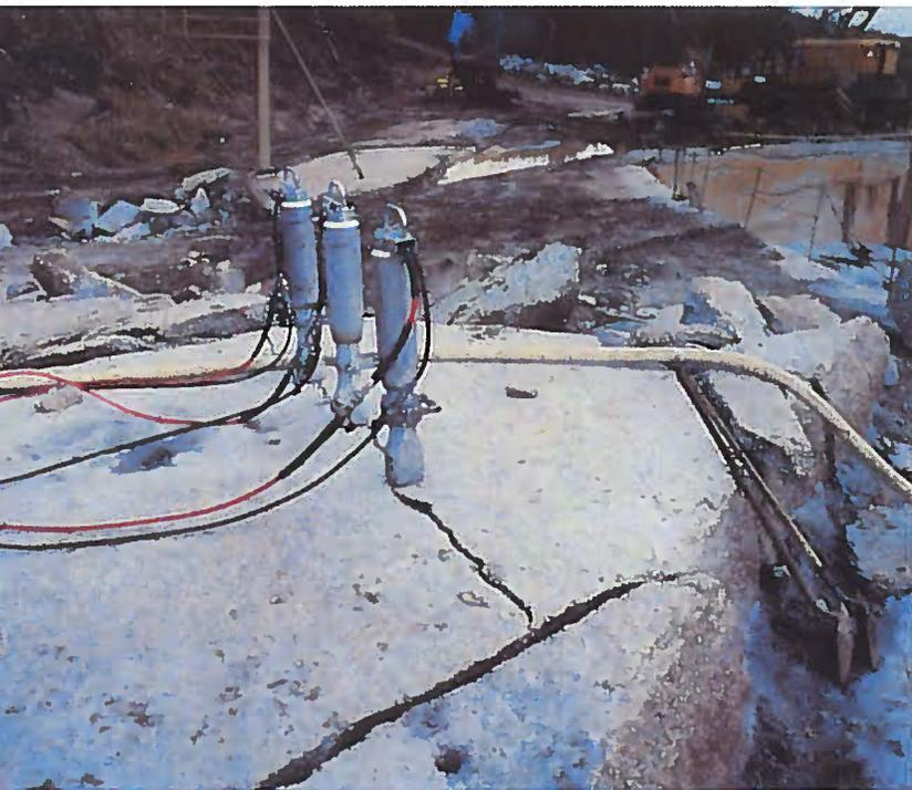
\*Three hydraulic splitters powered by a single pump generate over 2 million lbs. (1155 tons) of breaking force to split a 8 ft. x 22 ft. block of granite cap rock in a Midwest quarry. The Elco pump, with manifold, can power 4 splitters if more force is required.
