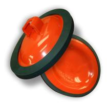
The Schmidt SureFit handway gasket simplifies installation of the handway cover. It eliminates loose gaskets that are difficult to keep properly aligned, make installation difficult and cause leaks. The SureFit gasket snaps onto the handway cover to ensure proper alignment and maximize a proper seal.
