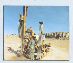
The CM-351 is a compact, powerful rig for drifter or downhole drilling of  $64\text{-}140\text{-}\mathrm{mm}$  ( $2\frac{1}{2}$  to  $5\frac{1}{2}$ ") blastholes. Fixed-length boom. Its 2.2-m (7'3") width makes it easy to transport.
