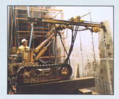
The LM-100 is ideal for small jobs in confined places; it makes fast work of holes 44-64 mm ( $1\frac{1}{4}$  to  $2\frac{1}{2}$ "). Compact, but uses a 3-m (10-ft.) rod change.
