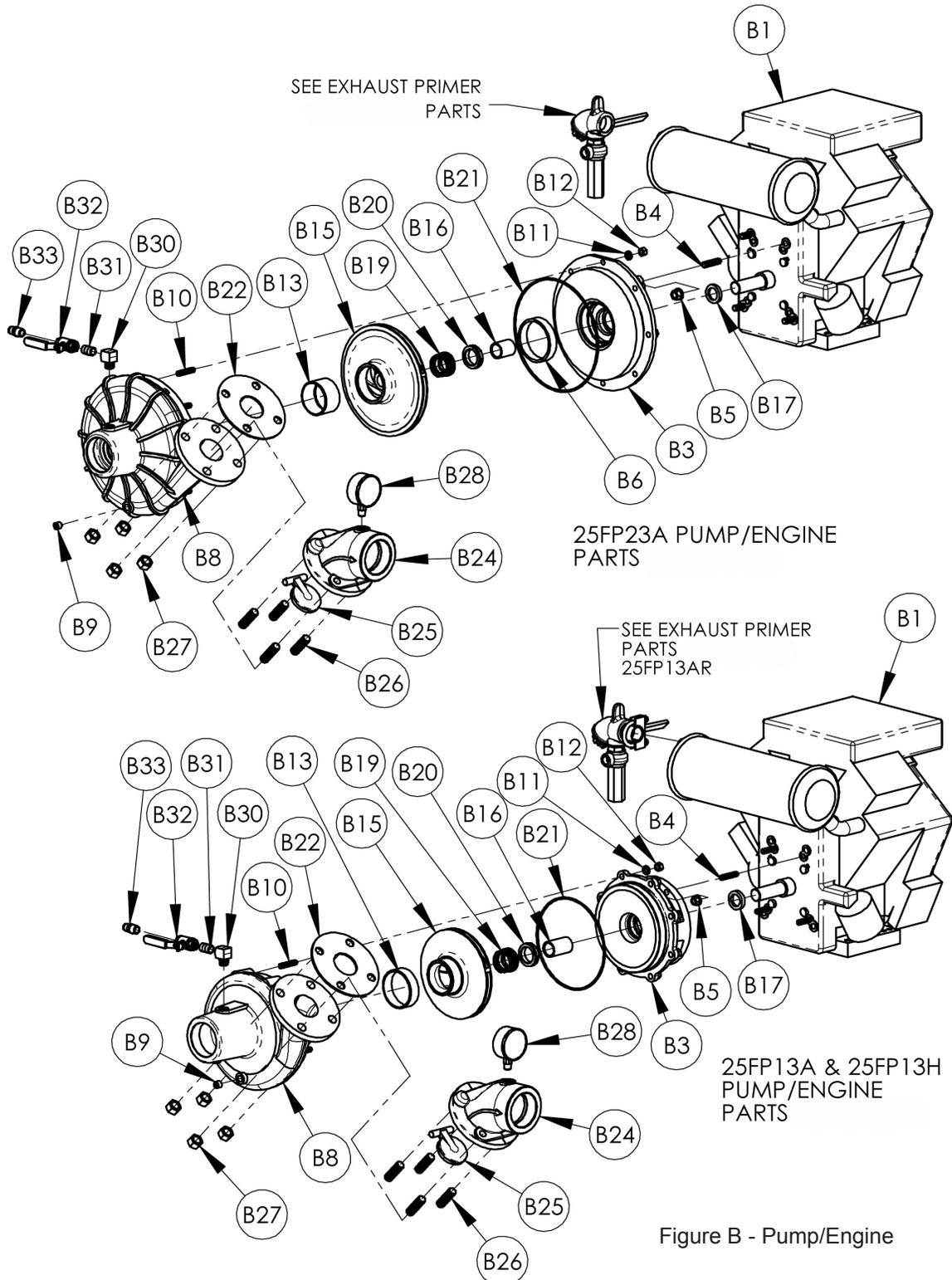
Figure B - Pump/Engine
